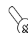
Bolt -4x12L, 2 EA :for Nozzle Holder -M4x12L, 2 EA :for Nozzle Holder, Gas Valve
