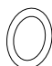
O-Ring -17.5 x 2.7T, 2 EA :for Gas Valve, 1 EA for Nozzle Holder, 1 EA
